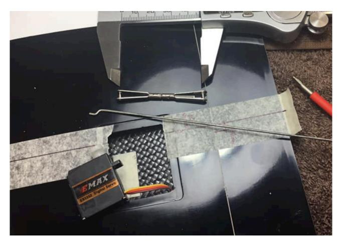
The elevator (no rudder on this 5 servo plane) is much more straightforward with a linear pushrod through the fuselage.
